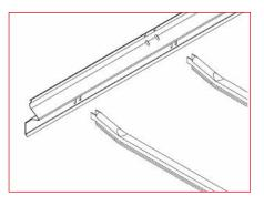
The special side profile allows a guide of the manure belt
