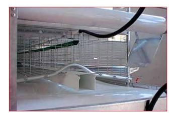
The solution with manure drying duct under the cage is ideal for moderate length sheds and allows to utilize the full cage depth. The special design with the duct all over the floor wire mesh grants a complete cleaning of the manure duct upper part done by the birds' feet.
