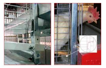
The egg saving baffle is designed to allow a firm grip of the birds' feet preventing accidental damaging of the eggs under it through accidental slipping.
