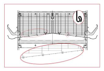
Thanks to its production technology Facco has designed the floor horizontal wire support as an extension of the partition wires thus granting a reduced sagging of the floors even when the is fully occupied thus preventing the concentration of eggs in the center of the cage. Its design facilitate the installation and through a proper distribution of the load ensures a longer lasting of the partition.
