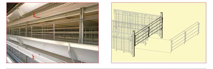
The sliding door is fitted on a special frame to ensure proper sliding while preventing unhooking.
