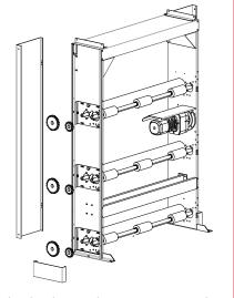
In the heavy duty manure removing unit steel sprockets ensures maximum durability and are designed to facilitate inspection and maintenance.
